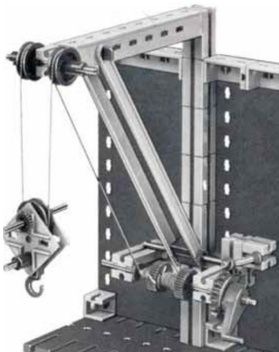
Abb. 14: Differentialwinde (aus: hobby2 Band 4 [3])
